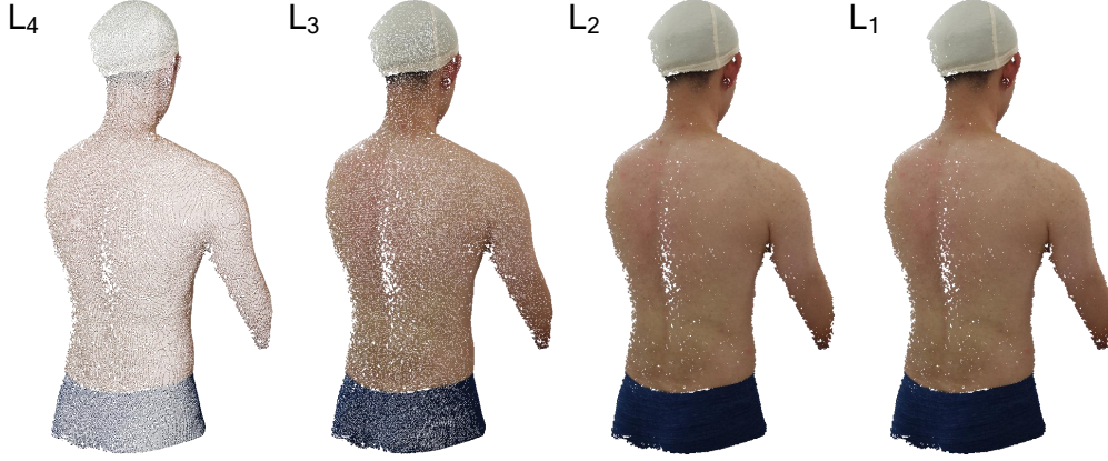
Figure 5: Point-clouds recovered from the hierarchical disparity images at 4 layers, starting from the coarsest layer L_4 ( 360 \times 480 ) to the finest layer L_1 ( 2880 \times 3840 ).
